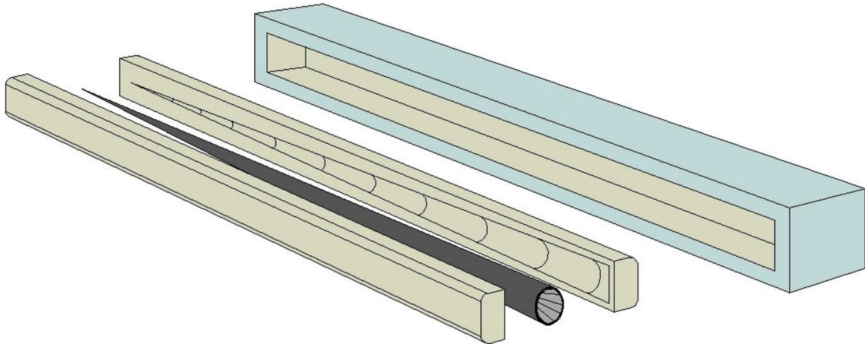
**Figure 3 Sled, Sabot & Projectile**
